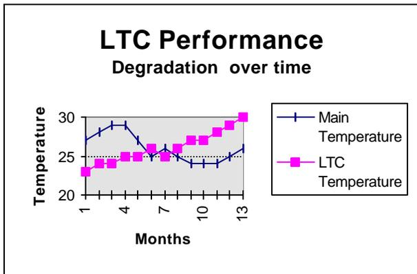
An instrument was installed that continuously monitors these temperatures. The benefits include longer duration between inspections, and improved diagnostics during operation and correlation to loading factors.
