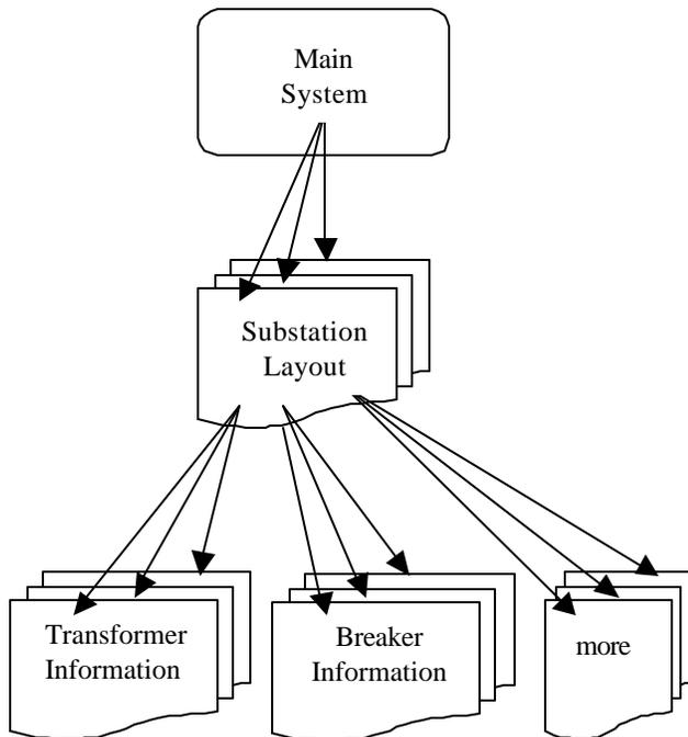
Each screen consisted of graphical objects representing items of equipment. To look at any item of equipment in more detail, the user simply pointed and clicked on the desired object. In this way the user could drill-down to any level of detail desired. The lowest level of detail for any equipment included:
